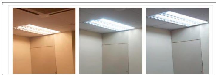
Fig. 1. Light setting of the Usability Testing Laboratory in MIMOS Berhad (a) 2700K; (b) 4000K (c) 6200K
