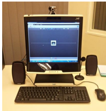
Fig. 2. Tobii Eye Tracker T60 used to capture fixation, heat maps and gaze plots [9, 14, 15]
