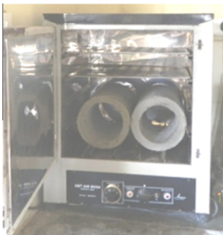
Figure 9 Pipe specimens placed in an oven.
