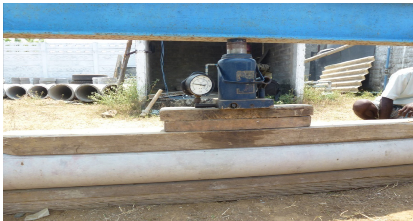
Figure 6 Specimen under three-edge bearing test.
