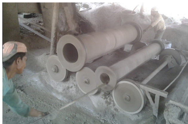
Figure 4 Pipe manufacturing process.
