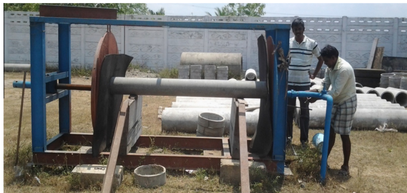
Figure 8 Specimen under hydrostatic test method.
