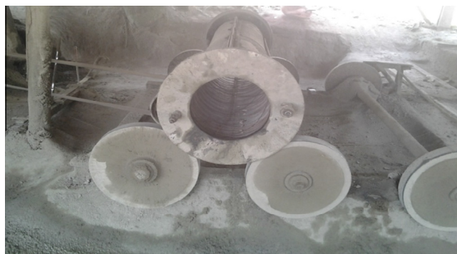
Figure 3 Pipe moulding machine.
