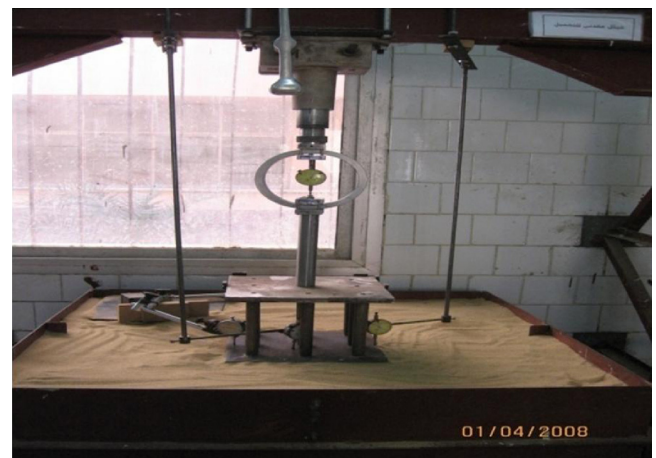
Fig. 5. Photograph showing loading cap and measuring devices.
