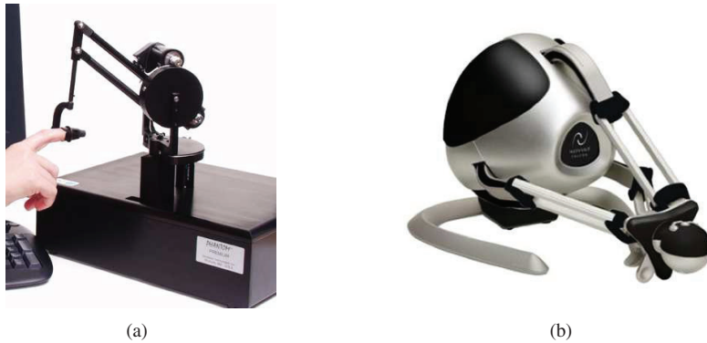
Fig. 1. Haptic devices: (a) The Phantom desktop from SensAble Technologies (six DOF) and (b) the Falcon from Novint (three DOF).
