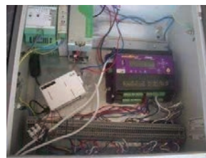
Fig4. Setup of the datataker and the Rpi inside the measurement
