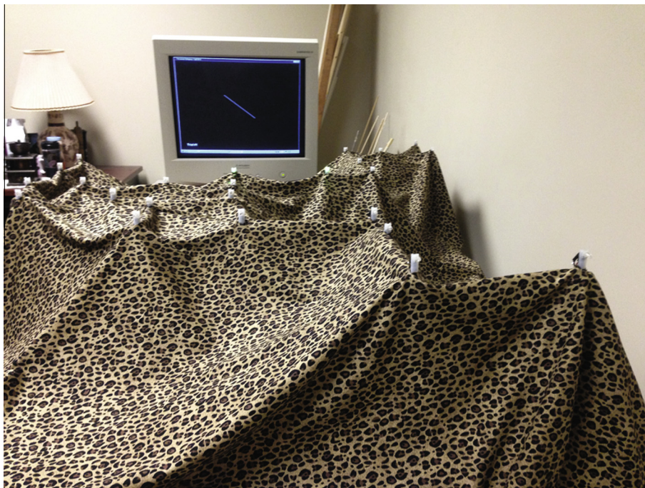
Fig. 1. A photograph of the horizontal and in-depth spatial intervals used as stimuli in the experiment. The endpoints of the spatial intervals that were judged are marked by light-emitting diodes (LED's), which were embedded within a textured surface. The adjustable line segment used in the matching task is visible on the computer monitor located behind the textured stimulus surface.
