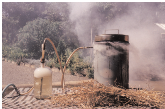
Figure 2: Apparatus for producing smoke-saturated water
