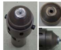
Fig. 1. Modular tool used during FSW trials
