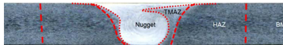
Fig. 11. Identification of the main different metallurgical zones on the FSW specimens in “as-welded” condition
