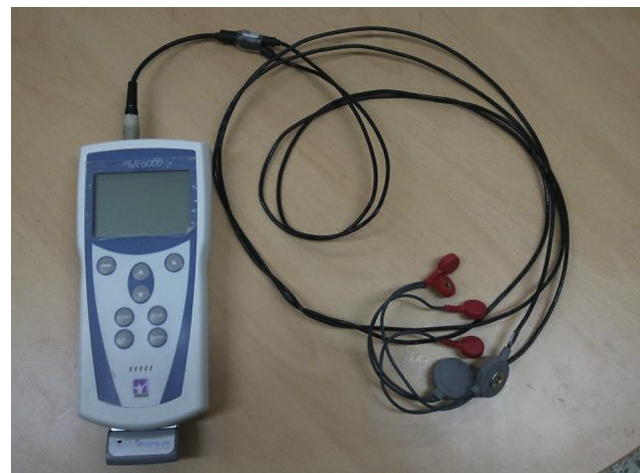
Figure 2 ME6000 electromyography system.
