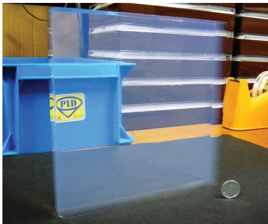
Fig. 6. Photograph of a large aerogel tile with n = 1.051 and \Delta_T = 40 mm. As a reference, the coin has a diameter of 2 cm.
