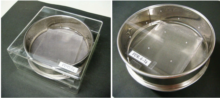
Fig. 1. Two types of pin containers: type-g (left) and type-a (right).
