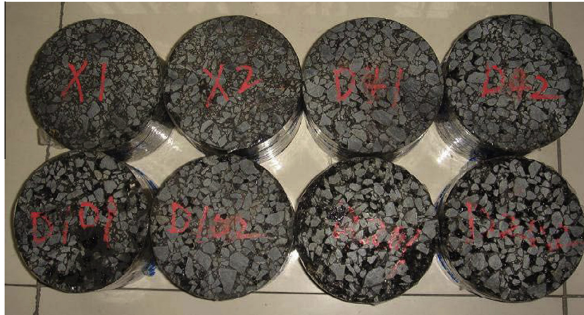
Figure 18. Indoor specimens for the small radius aggregates (X1 and X2) and single layer porous asphalt mixture (code starting with D).
