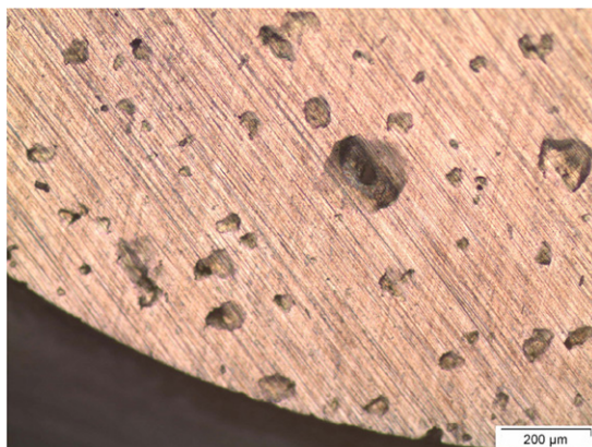
Fig. 2. Pitting corrosion after a polarization curve for the 304 stainless steel with original magnification of 100\times .
