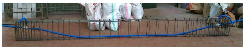
**Fig. 3** The prestressing strand placed inside the polyethylene duct.
