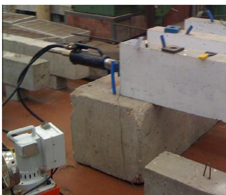
**Fig. 4** Application of the prestressing force.
