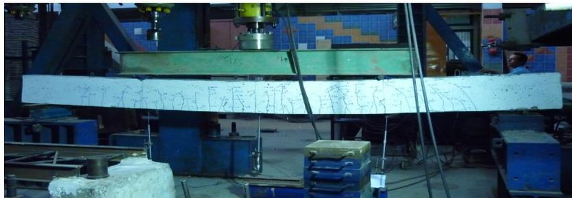
Fig. 7b Test set-up of beam specimens.
