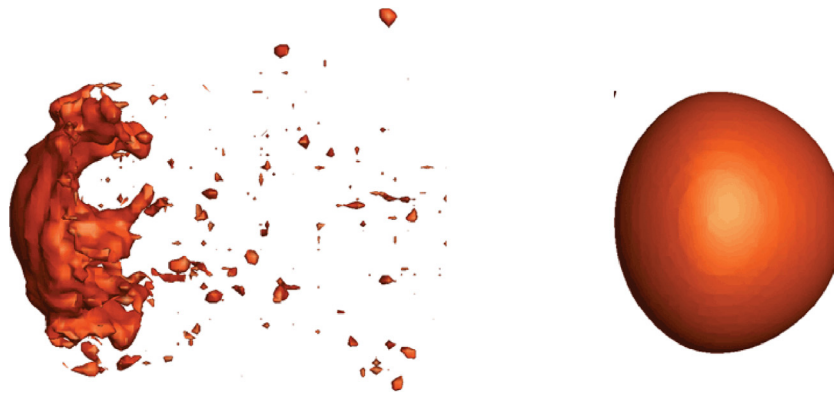
Fig. 3. (Left) Numerical droplet breakup at We = 3.4 with conventional discretisation (Right) Predicted droplet behaviour at We = 3.4 with liquid velocity extrapolation.
