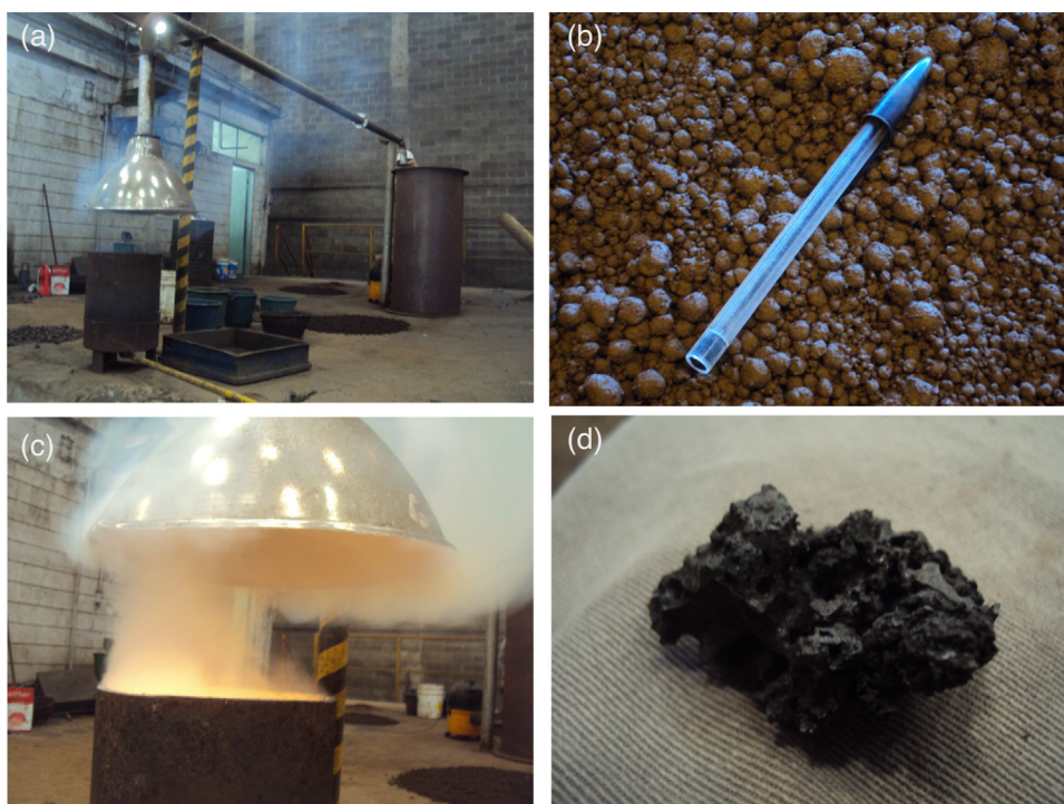
Fig. 2 – Pilot sintering plant upstream (a), with detail of the mixture (b), particulate material volatilized during the process captured by the hood (c) and pre-melting agglomerated – PCA (d). Author (2013).
