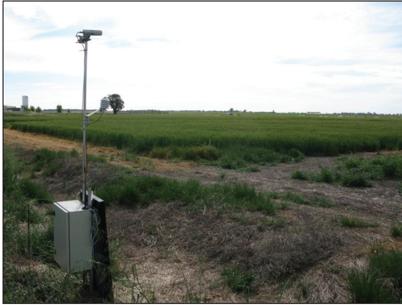
Figure 2. Photo of one of the eight CO 2 sensors at the AGFACE facility. The GMP343 is located at the top of the tower.
