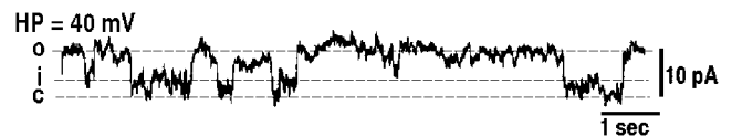
FIGURE 6 Unitary channel recording obtained in liposome-attached configuration of the patch-clamp technique. Shown is a representative current trace recorded at 40 mV (holding potential, HP ) from a patch containing one active channel under symmetrical conditions (150 mM KCl inside and outside the liposome). The open, intermediate, and closed states of the channel are indicated with dotted lines and the letters O, I, and C, respectively.
