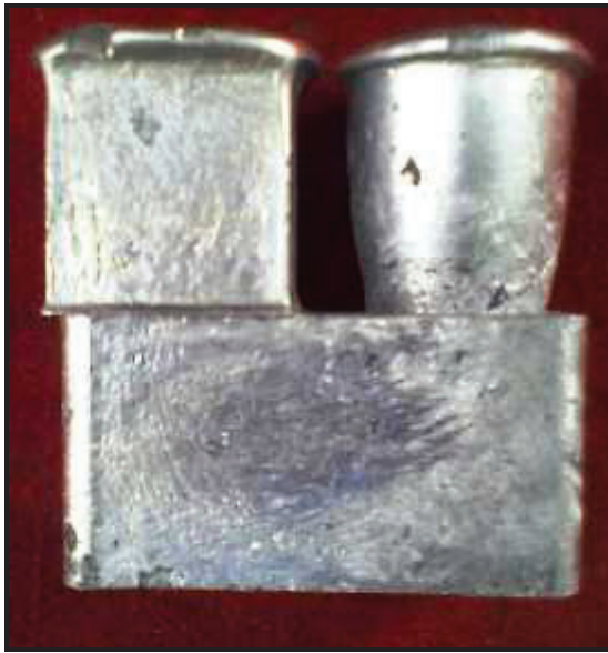
Fig. 1. A typical stir casted AA6061-B 4 C Composite
