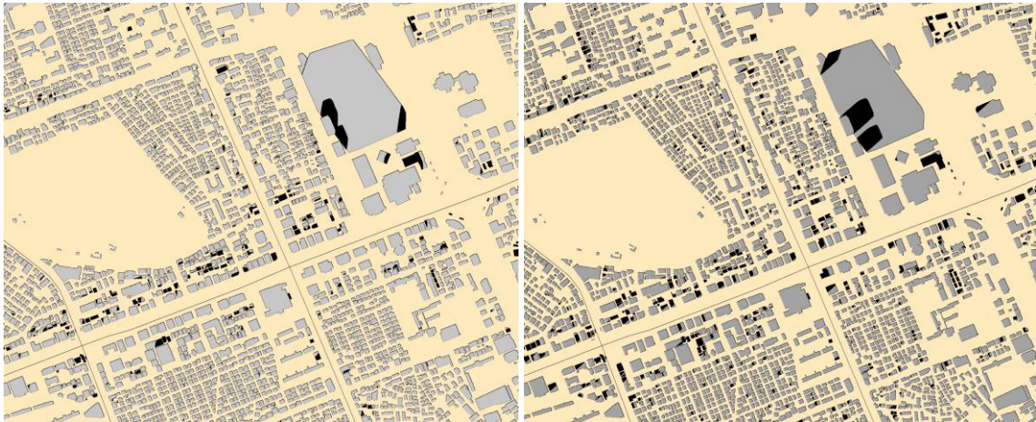
Fig. 1. The available rooftop area in Gangnam district on spring equinox at (a) 1PM (left) and (b) 3PM (right)
