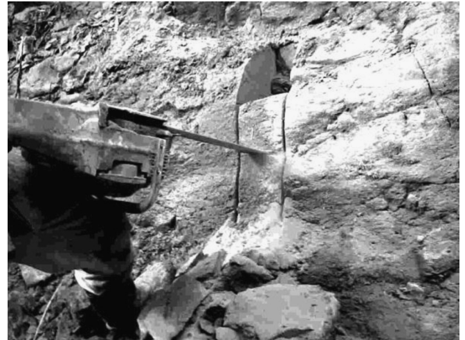
Fig. 19. Motor saw utilized to extract undisturbed soft rock blocks.
