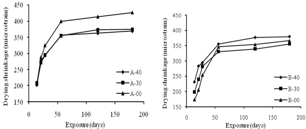
Fig. 2 Effect of fly ash on drying shrinkage in series A (left) and series B (right).
