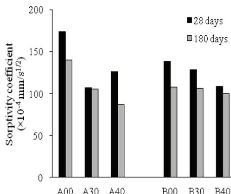
Fig. 3 Comparison of sorptivity coefficients.
