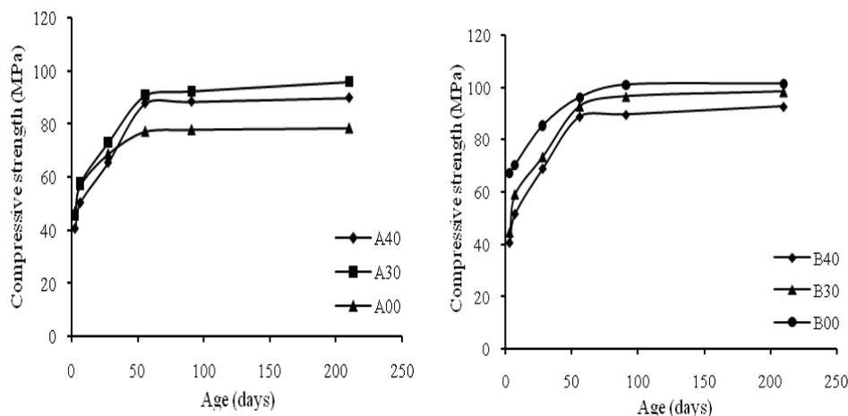
Fig. 1 Compressive strength development in Series A (left) and Series B (right).
