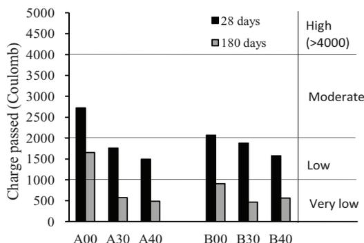
Fig. 4 Chloride permeability results.
