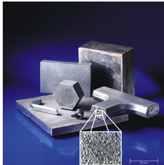
Fig. 3. Reference material: FOAMINAL® aluminum foam (closed cell porosity, closed surface skin).
