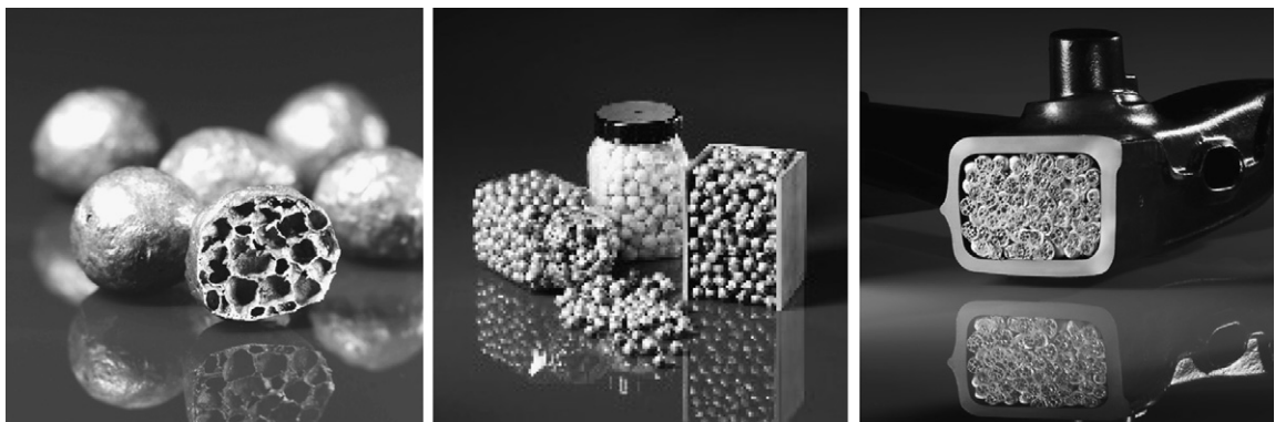
Fig. 1. Aluminum foam elements of approximately 10 mm diameter (left), foam elements and filled structure (middle) and cross section of automotive transverse control arm with aluminum foam–polymer hybrid core (right).
