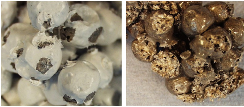
Fig. 10. Failure of adhesive bonding (left; PA; b/D = 5 \times 10^{-3} and b/D = 15 \times 10^{-3} ) and rupture within the aluminum foam element volume (right; EP; b/D = 10 \times 10^{-3} ).
