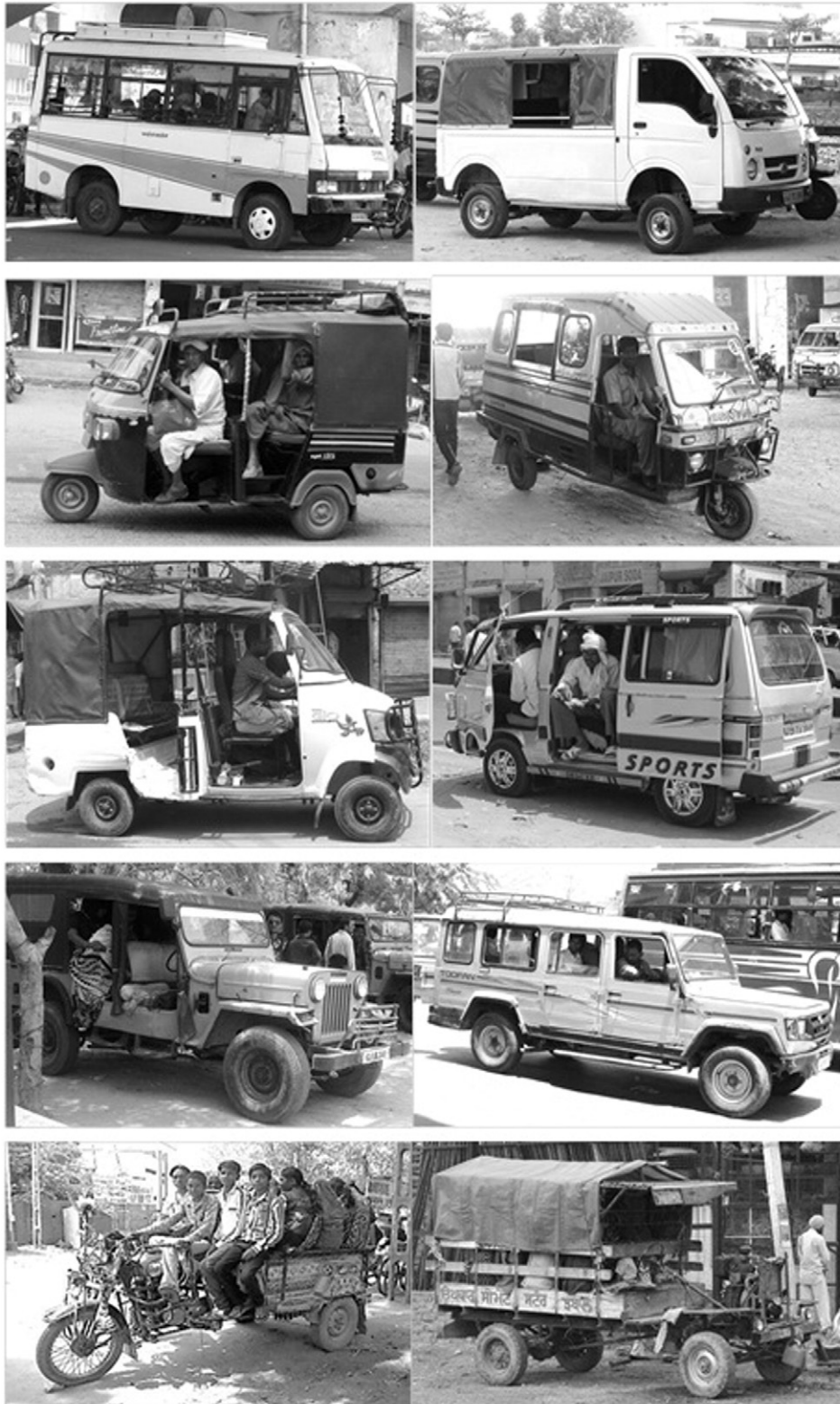
Fig. 1. Photographs of typical informal public transport modes studied in the target cities/city regions (Left to right, top to bottom: Minibus, Tata Magic , Auto-rickshaw, Vikram , Mahindra Gio , Maruti Omni , Jeep , Force Cruiser , Chakda , Kaduka ). Source: Photographs taken by the study team during field visits.
