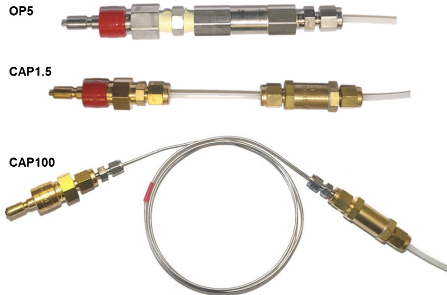
Fig. 1. Assembly of the three flow restricting apparatus investigated. Each apparatus comprised: OP5; quick connect stem, orifice plate, 2 \mu\text{m} particle filter, reducing union, sampling tube. CAP1.5; quick connect stem, tube containing a 1.5 cm crimped capillary tube, 15 \mu\text{m} particulate filter, sampling tube. CAP100; quick connect stem, reducing union, 100 cm capillary tube, reducing union, 15 \mu\text{m} particulate filter, sampling tube.
