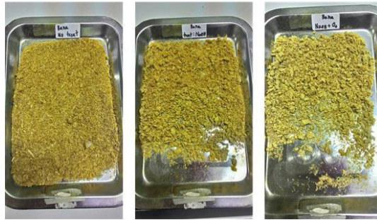
Fig. 1. (a) Untreated material; (b) Elephant grass after alkali pretreatment; (c) Elephant grass after ozonolysis process.
