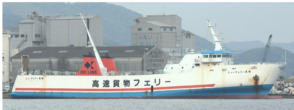
Fig. 11. New Ferry Misaki (68.0 m (Lpp), 12.3 m (Bmd), 8.95 m (Dmd), 3.2 m (draft), 4076 ps (power)). (Courtesy of Hirofumi Morieda).
