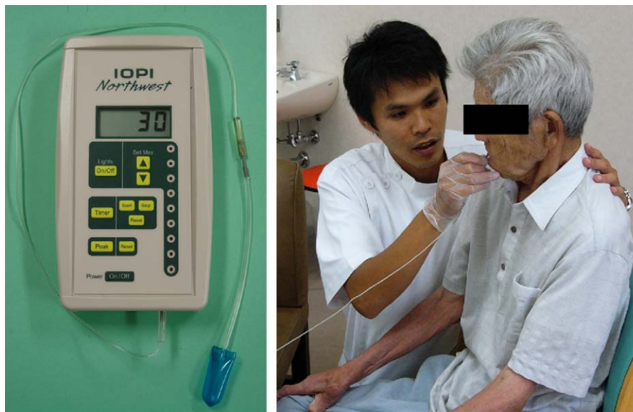
Figure 1 Iowa oral performance instrument (IOPI, left), and its usage in the measurement of maximum tongue pressure (right). (Through the courtesy of Prof. Isami Kumakura, Kawasaki University of Medicine and Welfare.)
