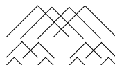
Fig. 7. The figure shows the resulting (Hermitian transposed) Cooley–Tukey FFT factorization for the matrix F_8 P_8 .
