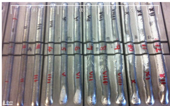
Fig. 7. Morphology of tracks produced with combined wire and single powder delivery. PFR: (a) 2.0 gmin -1 , (b) 3.2 gmin -1 , and (c) 4.8 gmin -1 .
