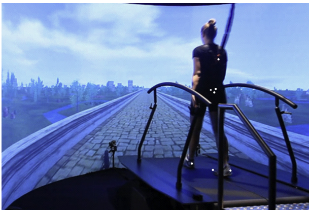
Fig. 1. Gait Real-time Analysis Interactive Lab (GRAIL), consisting of a dual-belt instrumented treadmill placed in a speed-matched virtual environment with 180^\circ projection. An optoelectronic system with reflective markers was used to measure joint movement.
