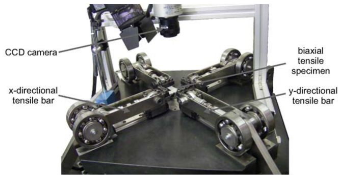
Fig. 1. Biaxial tension test according to Merklein and Biasutti [12].
