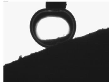
Figure 2: A drop of \text{scCO}_2 generated from a capillary tube is brought into contact with a porous plate substrate angled at 21^\circ . The bulk phase is de-ionized water ( P = 48.9 \text{ MPa} ).
