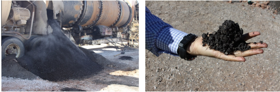
Fig. 2. 100% millings after adding 1% emulsion.
