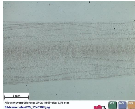
Figure 11: Cross section, solidification lines
