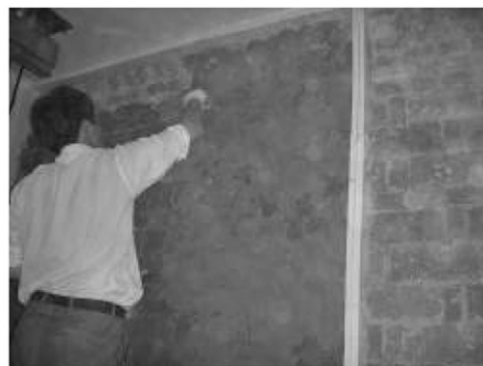
Figure 12 Pouring of foam concrete into the voids of the test wall panel, and the application of inorganic stucco system.
