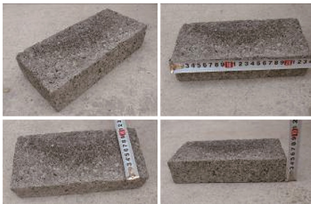
Figure 4 Brick masonry made of industrial solid wastes, cement, and water.
