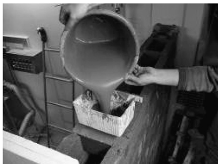
Figure 12 Pouring of foam concrete into the voids of the test wall panel, and the application of inorganic stucco system.
