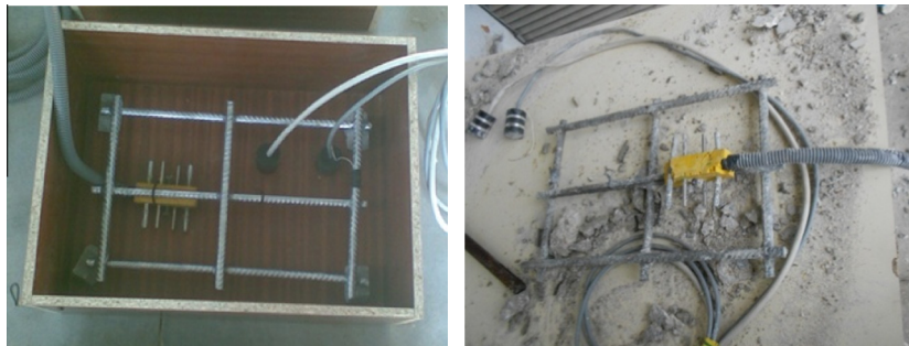
Fig. 2. View of the placing of the Moncorr and Conduclcorr monitoring systems before the casting of the test prisms and after 700 testing days.
