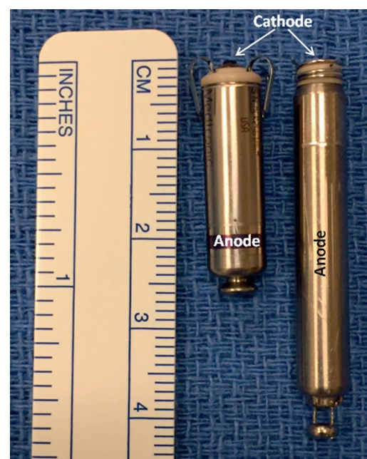
FIGURE 2 The Single-Component (Fully Self-Contained) Leadless Pacemakers
