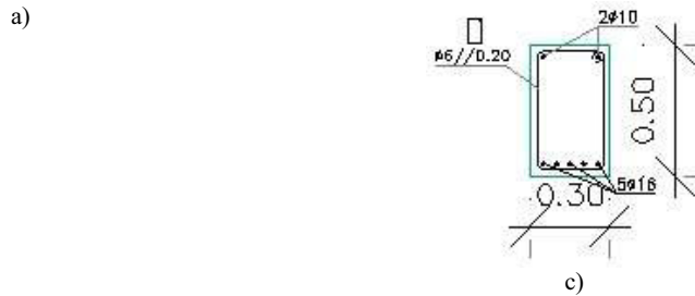
Fig. 2. Infilled RC frame specimen dimensions a) general dimensions b) columns and b) beams dimensions and reinforcement detailing.
