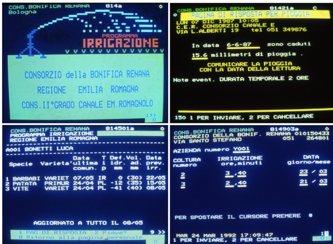
Figure 1: Videotext pages of irrigation scheduling service (1984), with input videotext page to communicate the meteorological data measured by the farmers (pluviometer) and with information on irrigation depth and length of run.
