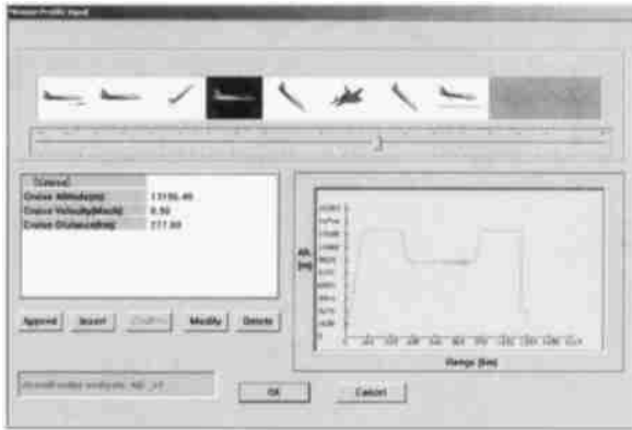
Fig. 3 Interface of mission profile input boundary could be computed [9, 12] and the designer could control whether to display it or not; if unusable, EDRIPS will show prompts through the interface or pop-up dialogs. The designer could use his mouse to pick up a feasible design point in the solution space formed by different boundaries and view the values of T_{SL}/W_{TO} and W_{TO}/S of it in real time. As an assistant measure to make the selection more reasonable, the design points of existent aircraft that belong to the same category with the current design could be displayed in the constraint diagram as references.
