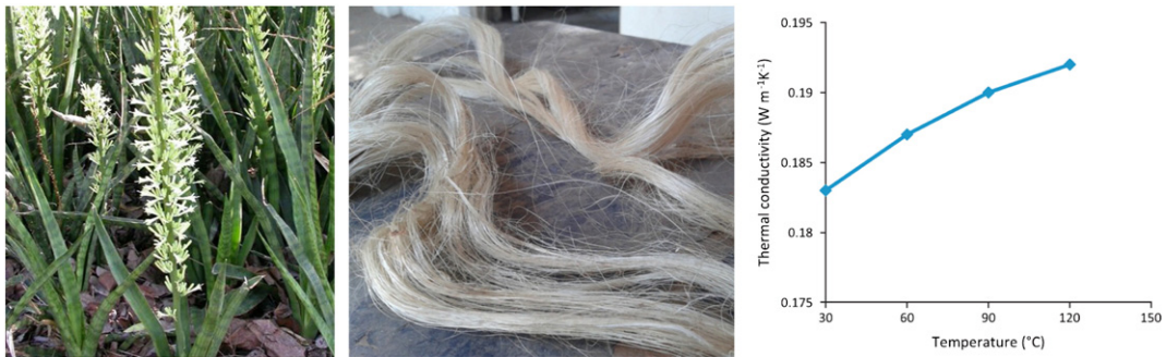
Fig. 13. Sansevieria plant (left) and fiber (middle). On the right, thermal conductivity trend vs. temperature measured in [78].
