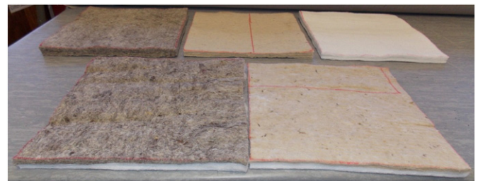
Fig. 17. Samples made of recycled PET tested in [93].
