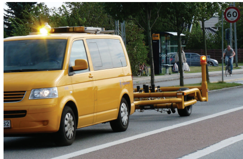
Fig. 1. The open trailer ‘decibella’ applied by the Danish Road Directorate for its CPX noise measurements
