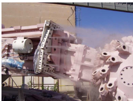
Fig. 1. Air-and-water spraying curtain in a roadheader (Libera et al. 2010)
