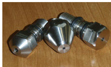
Fig. 2. STK air-and-water spraying nozzles (Prostański 2011b)
