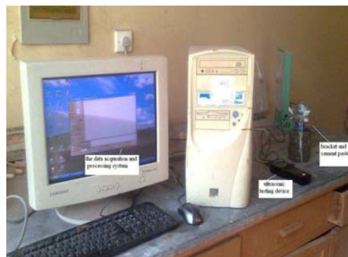
Fig. 1. The real-time ultrasonic monitoring device for concrete early age shrinkage
