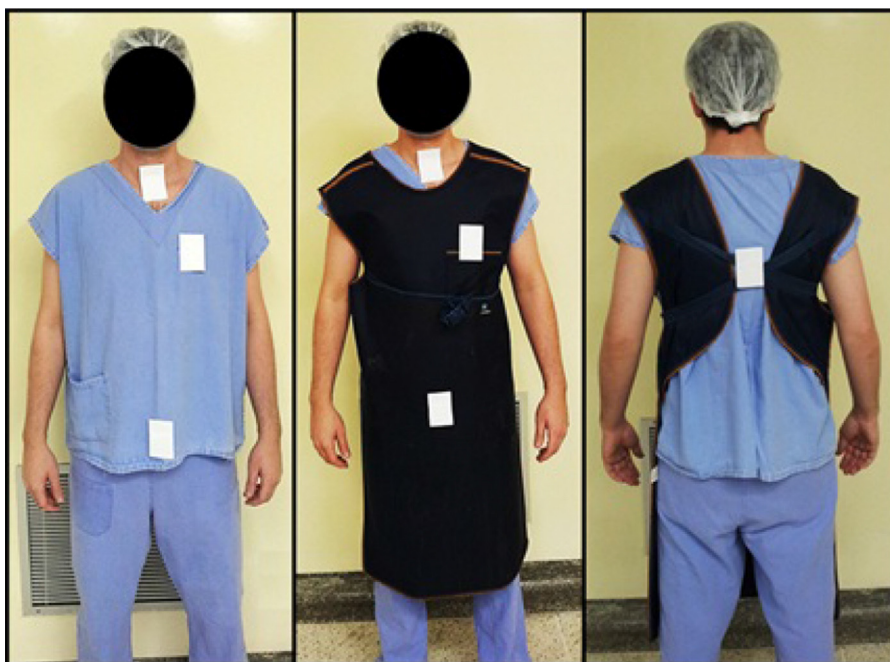
Fig. 2 – Anterior and posterior locations of the dosimeters on the team members (above and below the lead protector).
