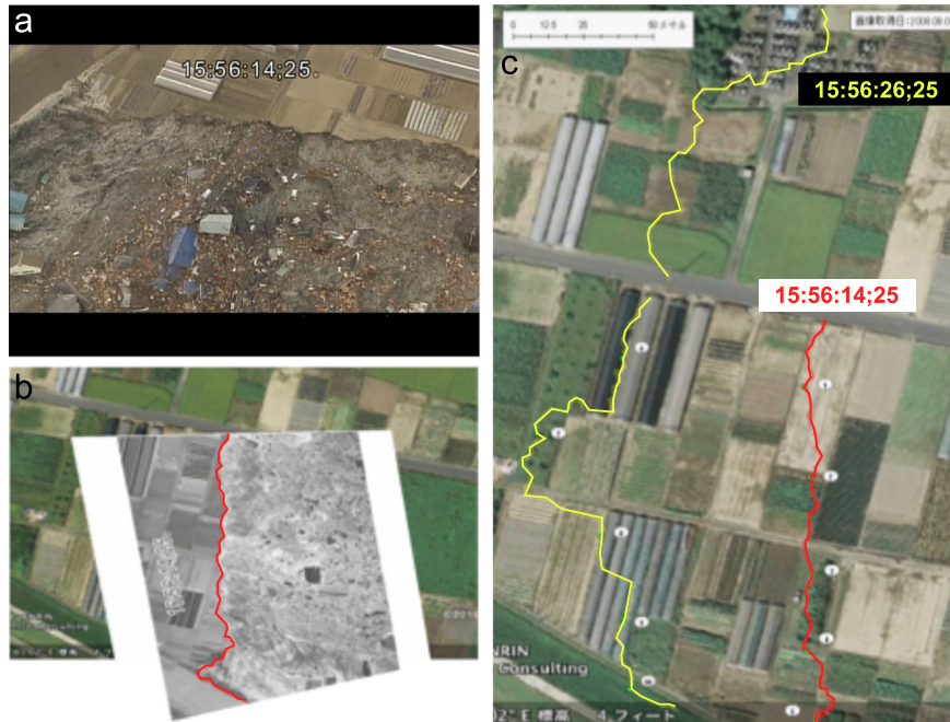
Fig. 6. Procedure of capturing tsunami front from the video. (a) A frame divided from the original video at 15:56:14 (Hours:Minutes:Seconds, 11 March 2011, JST). (b) Result of projective transformation of the captured image. (c) Result of mapping tsunami front captured from the video.
