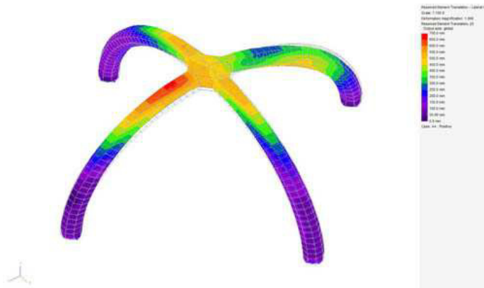
Fig 14: Typical Primary Tube Analysis (Image by Barton Engineers)
