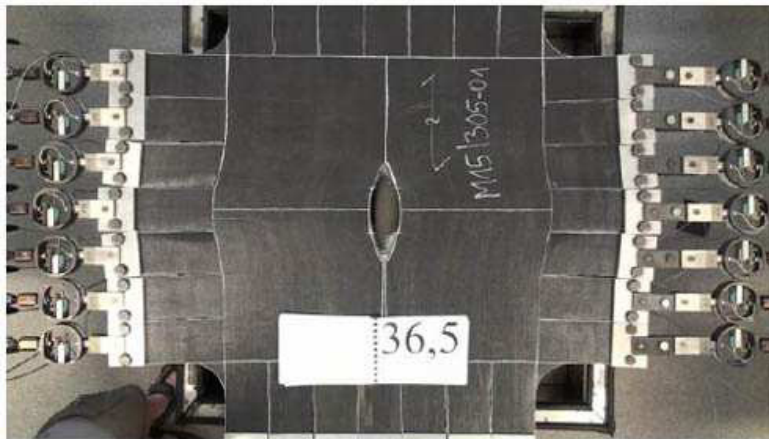
Fig 13: Wide Panel Tear Test on Coated Polyester Fabric (Image by DEKRA)
