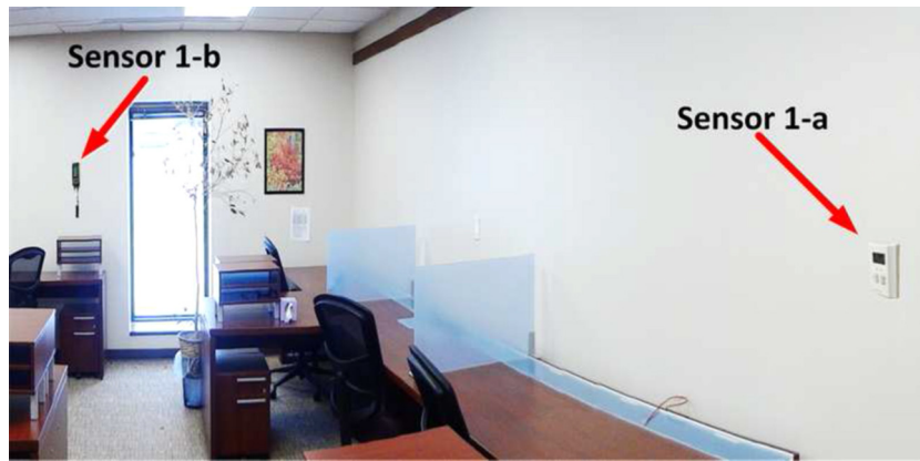
Fig. 1. Location of the temperature sensors in the test-bed. The sensor 1-a is the room temperature sensor and the sensor 1-b is a temperature data logger installed to calculate measurement errors.
