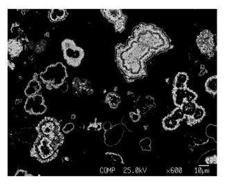
**Fig. 1.** Backscattered electron image (COMP, compositional contrast) of a polished block of the ITO powder. The image shows ITO particles (bright) embedded in epoxy resin (dark) and polished to a flat surface. Particle outlines represent transects through individual particles. Particles are generally rounded aggregates of hollow spheres with high surface to volume ratios. The scale bar is 10  $\mu$ m.
