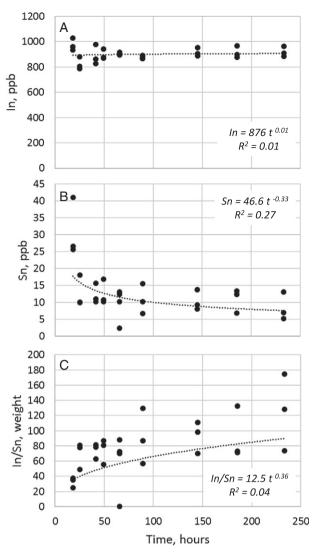
**Fig. 5.** Concentrations of In (A) and Sn (B) and the In-Sn ratio (C) measured in the simulated stomach acid (the PBET solution) in contact with ITO powder. In and Sn display strong positive correlations with time. This environment is not particularly selective in the dissolution of In and Sn.
