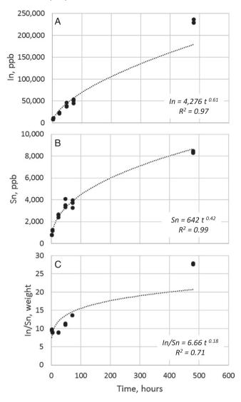
**Fig. 4.** Concentrations of In (A) and Sn (B) and the In-Sn ratio (C) measured in simulated deep lung fluids (the ALF solution) in contact with ITO powder. In and Sn display strong positive correlations with time. The evolution in In/Sn demonstrates selective dissolution of In.
