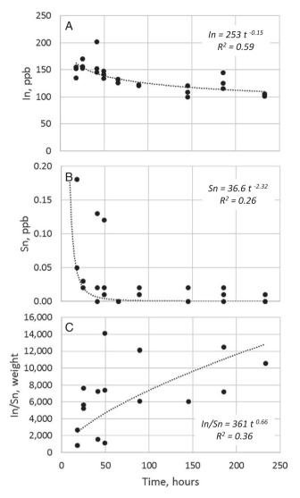
**Fig. 2.** Concentrations of In (A) and Sn (B) and the In-Sn ratio (C) measured in deionized water in contact with ITO powder. The negative correlations of In and Sn with time are likely to be caused by sorption of metals to the container walls (Robertson, 1968; Smith, 1973).
