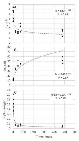
**Fig. 3.** Concentrations of In (A) and Sn (B) and the In-Sn ratio (C) measured in simulated upper respiratory tract fluids (Gamble's solution) in contact with ITO powder. As for Fig. 2, the negative correlation of In with time is likely to be caused by sorption to the container walls. The substantial decrease in In/Sn over time is a combined effect of In removal and Sn dissolution.
