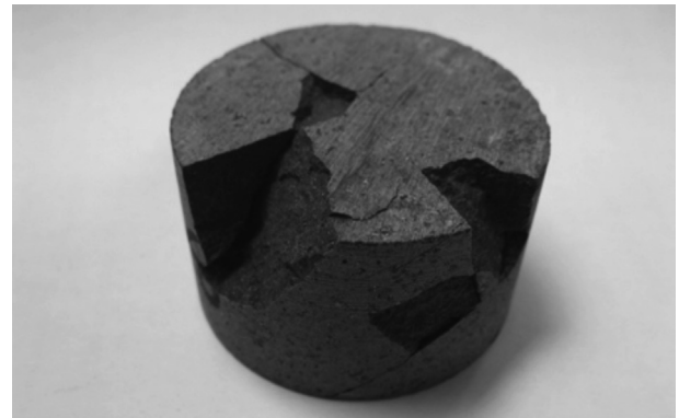
Fig. 9. Basalt #1 showing surface spalling after microwave treatment for 35 s at 3 kW power.
