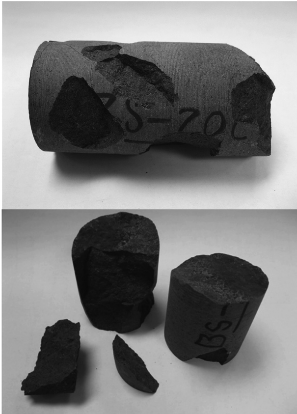
Fig. 11. Basalt #1 cylinders burst after microwave treatment for 120 s at 3 kW power.
